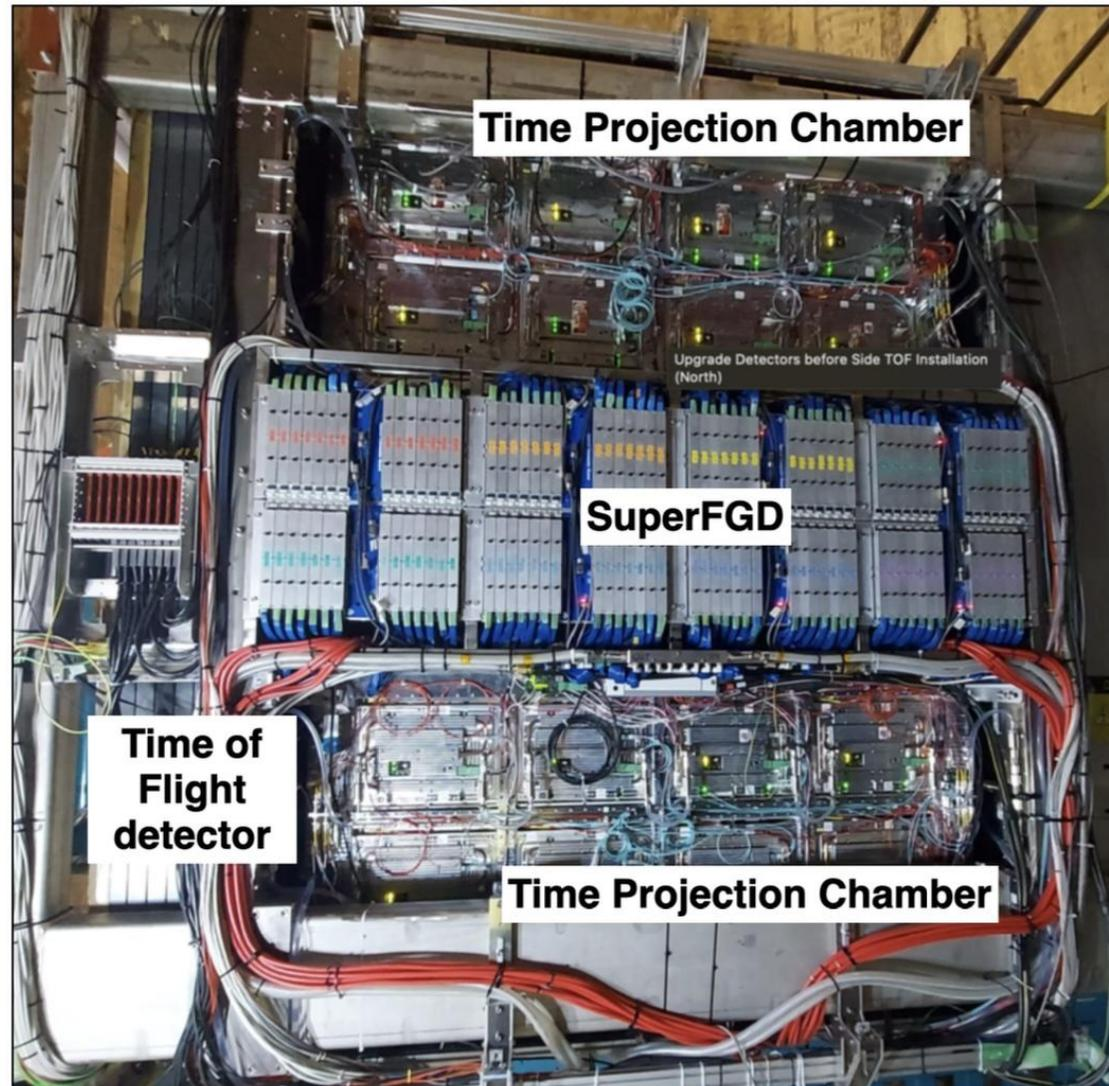
Installation of all detectors (SuperFGD, HA-TPC, TOF) into ND280 magnet completed in May 2024
