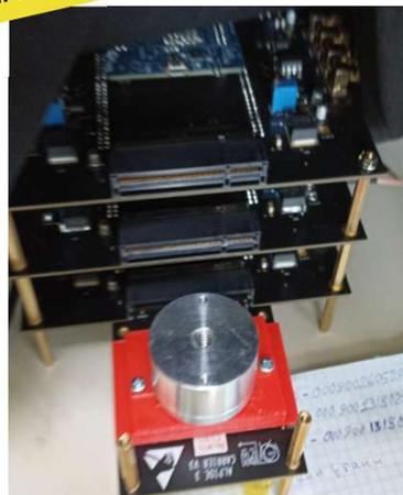
$^{55}\text{Fe}$  source with Aluminum collimator
