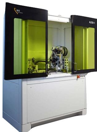
Chips alignment and gluing
