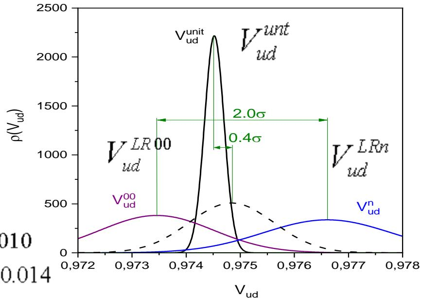
$$V_{ud}^{nLR} = V_{ud}^{n(V-A)} \times \sqrt{\frac{1 + 3\lambda_{n,V-A}^2 [1 + (\delta^2 + \zeta^2) + 2 \frac{(3\lambda_{n,V-A}^2 - 1)}{(3\lambda_{n,V-A}^2 + 1)} \delta \zeta]}{1 + 3\lambda_{exp,LR}^2 (1 + \zeta^2)}}$$
