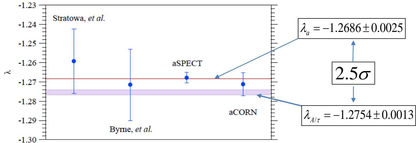
FIG. 10. A summary of the results for  $\lambda = G_A/G_V$  from neutron  $a$ -coefficient experiments. The horizontal line is the weighted average:  $\lambda = -1.2686 \pm 0.0025$ . The shaded region shows the 2022 PDG recommended value  $\lambda = -1.2754 \pm 0.0013$ .
