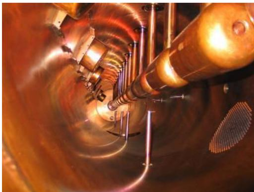
**Inside Drift Tube Tank**
