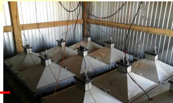
12 former KASCADE-Grande scintillation counters with  $S=0.64 \text{ m}^2$  in surface part of 19 station
