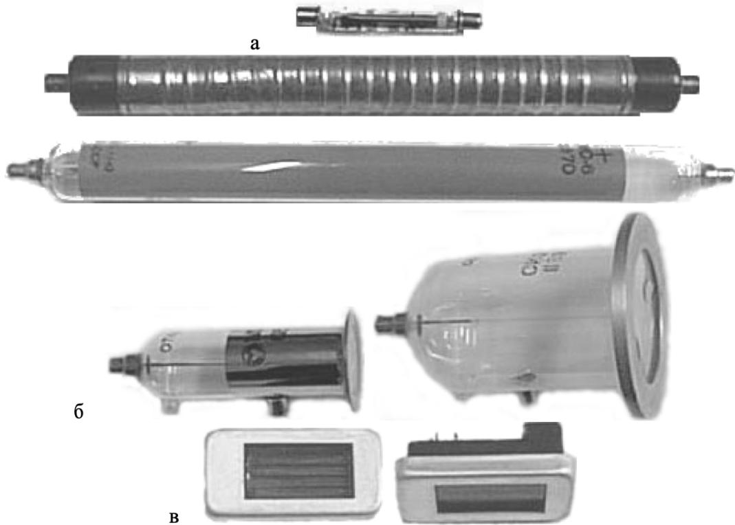
Figure 3.3: Geiger-Müller Counters. a – cylindrical, b – end-window, c – pancake
